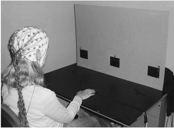
Fig. 1 – Stimulus setup used in this study. Sounds were presented from any one of three loudspeakers. The squares located above each loudspeaker indicate the fixation point (above the central loudspeaker) or the goal locations for leftward or rightward saccades (above the left and right loudspeakers). The response key was aligned with the central loudspeaker.
